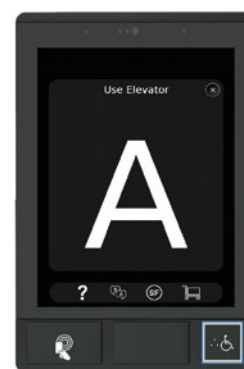
Elevator assignment and audible announcement regarding assignment and location of the elevator
