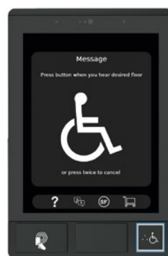
Audible explanation of how to use function and listening in ascending order of the landings for destination floor selection
